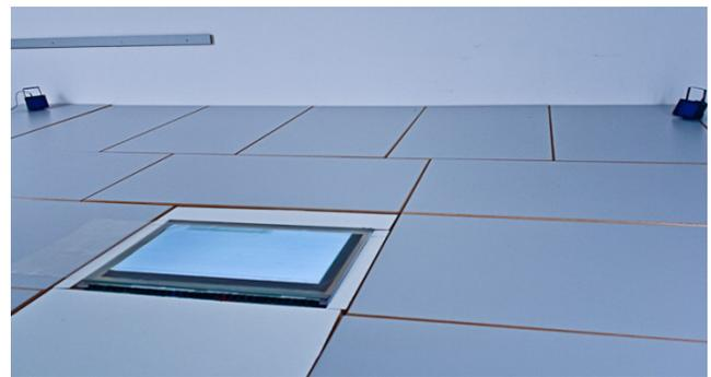
Figure 5: (a) On our current working prototype only a sub-region is interactive (projection screen, compliant surface and one floor tile removed).
