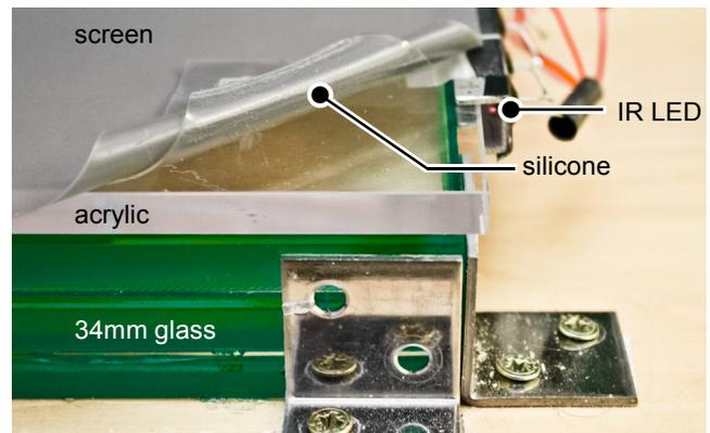
Figure 4: We use 34mm safety glass, 8mm acrylic, *Tectosil 185* silicone, and *Rosco* projection screen.
