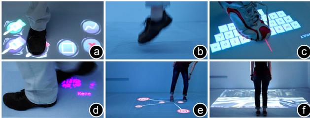
Figure 2: (a) Users trigger interactions with a specific foot posture, (b) invoke menus by jumping, (c) interact precisely using a hotspot, which is (d) enabled by sole-based user recognition. (e) FTIR-based tracking also allows controlling applications using body posture and (f) foot posture.
