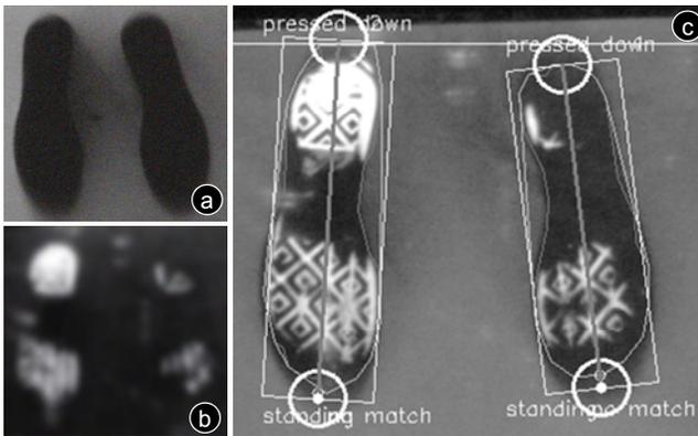
Figure 3: A user wearing shoes with black soles is standing on our floor prototype. (a) Front DI, (b) FTIR, (c) Front DI with FTIR, at 1mm resolution camera.
