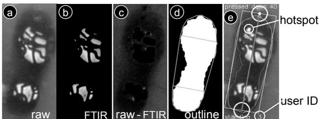
Figure 17: Sole processing (a) raw image, (b) thresholding extracts FTIR, (c) DI = raw minus FTIR, (d) Thresholding (blur(DI)) with convex hull and widths, and (e) annotated.
