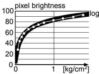
Figure 19: We found the brightness response of our stack-up to be roughly logarithmic with pressure (acrylic waveguide with Tectosil 500 silicone and Rosco projection screen)
