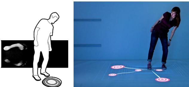
Figure 21: Sensing pressure using FTIR enables fish tank VR (here uses front projection).
